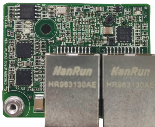
Figure 1-1 Appearance of the MD500-EN1 card
