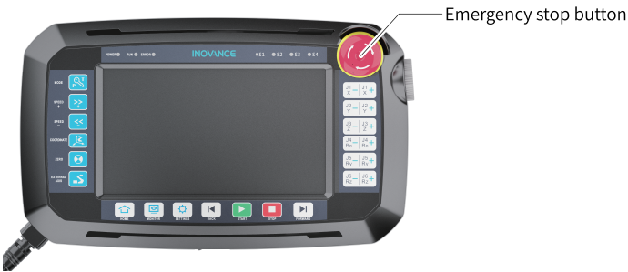
Figure 2-1 Teach pendant emergency stop button
