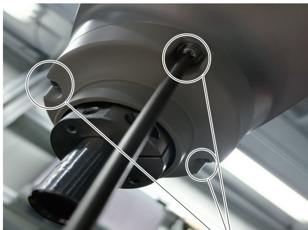
Screw at spline nut enclosure bottom Three M4x10 cross flat elastic integral screws
